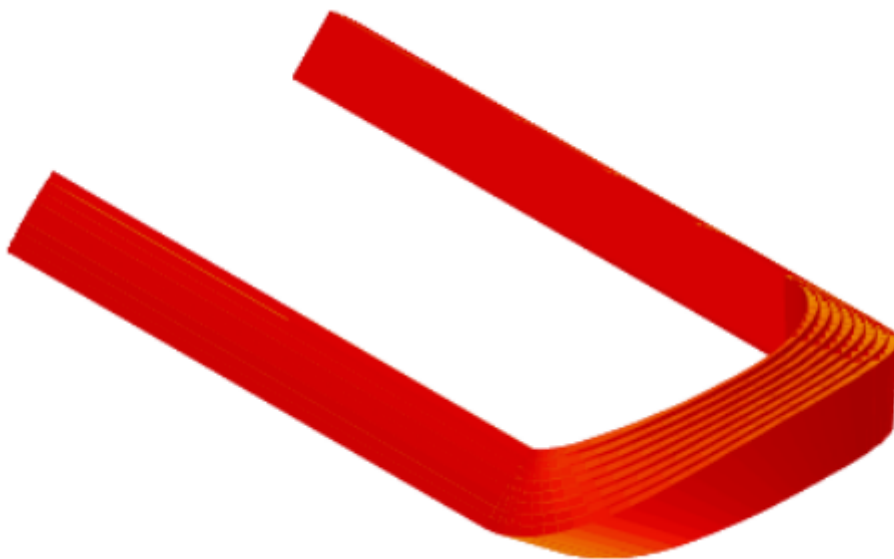
Fig. 11.18: Coil end design with differential geometry methods.
